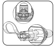
11. Assemble the valve insert with the new lever and lever support.
