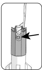
**IMPORTANT!** Never angle the lever more than 50 degrees as this may damage the contact surfaces on the lever support. When the valve insert is mounted in the breathing valve housing, the lever is prevented from angling more than 50 degrees. When the valve insert is removed from the breathing valve housing, the lever can be angled more than 50 degrees and thus damage the lever support.
