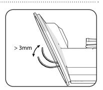
17. Use the lever bar to make sure that the lever is in the correct height. The lever must be in the upper area of the lever bar.
