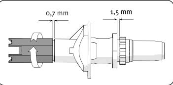
10. Mount the lever in the lever support with the pin in one of the deep slots. Check that the bend ends up in the right direction according to the rounded side of the valve insert.
