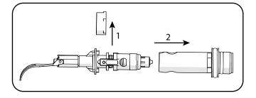
4. Press together the valve insert by hand so that the pin can fall out.
