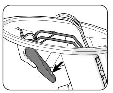
16. Make sure that the lever has a resistless movement of at least 3 mm.
